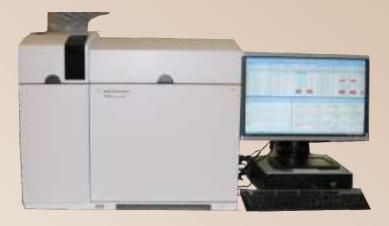
Spectro owns this high-tech instrument for fulfilling the requirements of their esteemed customers. We have ICP-MS Make: Agilent Technologies, Model: 7700 Series, G5700A
