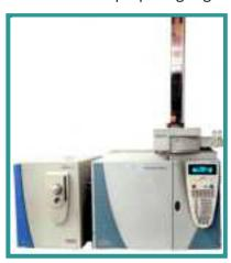
Spectro possess Gas Chromatography-Flame Ionization Detector to analyze the presence of trans-fatty acids in different Food products. We have all the facilities to test Food products (raw or cooked) to carry out several Physical, Chemical & Microbiological tests.
